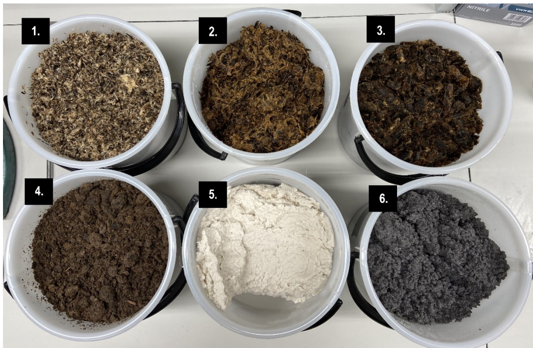
Figure 6. The analyzed samples of fibre-rich side streams included 1) knot reject, 2) screening reject, 3) knot washing reject, 4) fibre sludge, 5) fibre clay, and 6) deinking sludge.
