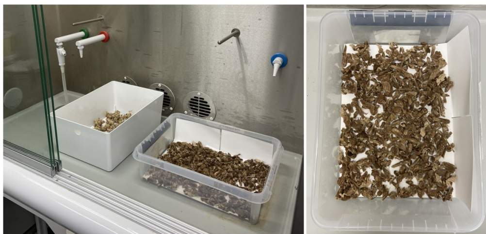
Figure 7. Example of the drying set-up. The samples were air dried in separate plastic containers in a fume hood.
